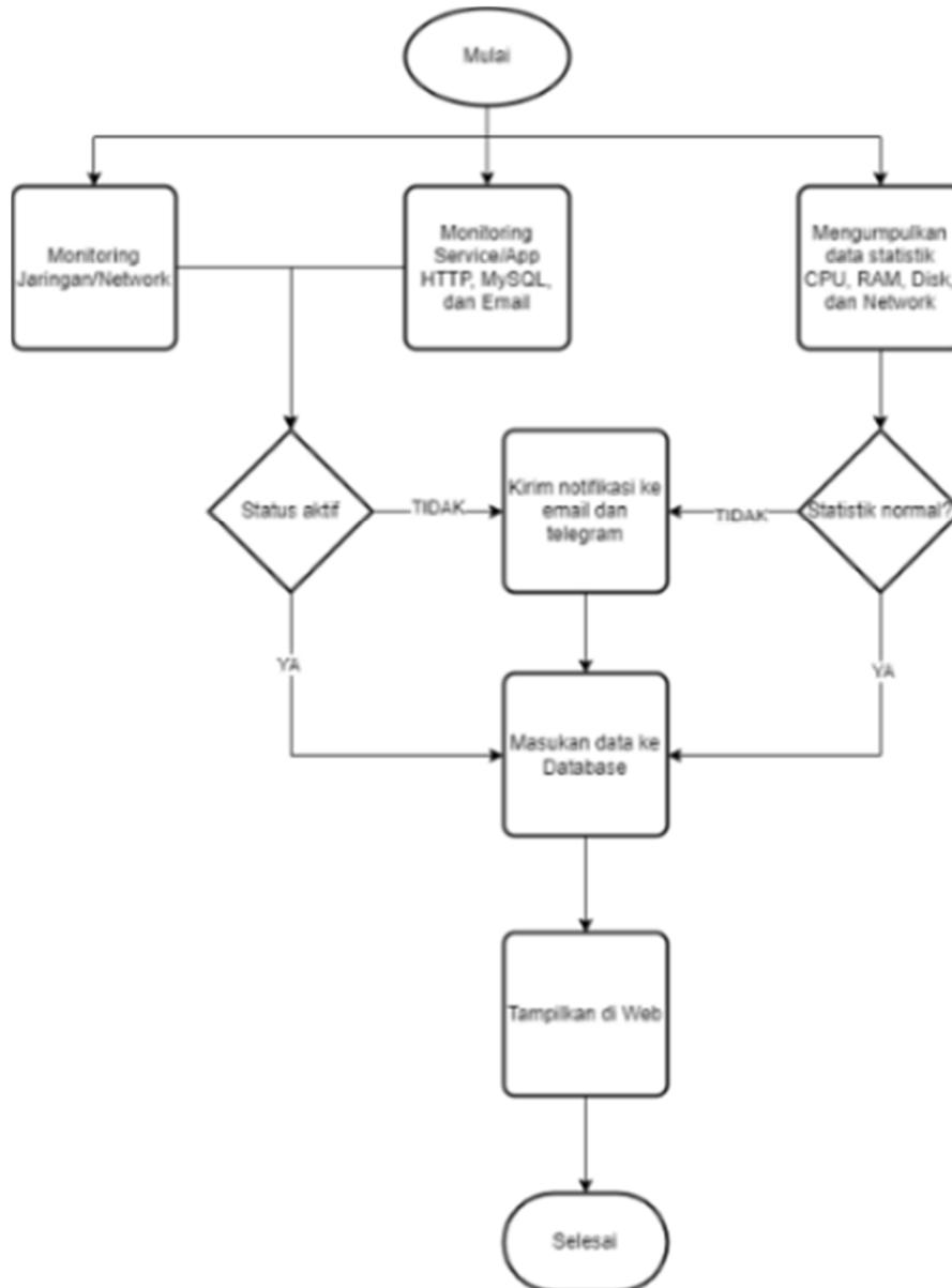
Gambar 2. Flowchart Sistem Monitoring Baru
